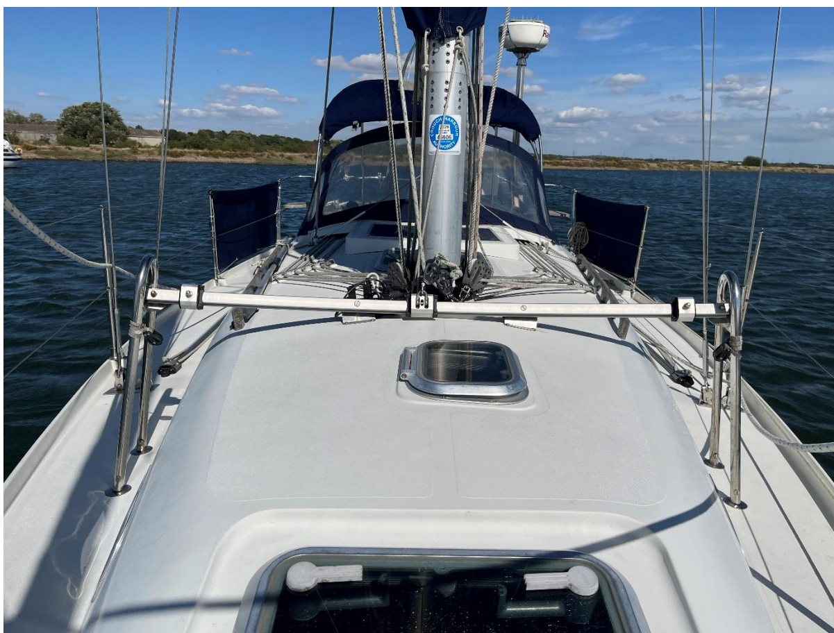
Self Tacking jib track, the small hatch is above the WC compartment
